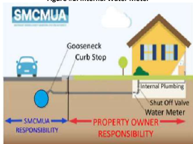
Figure #1: Internal Water Meter
