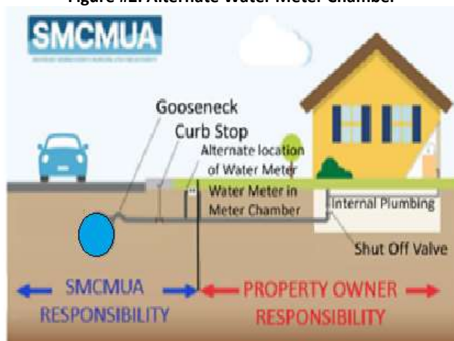
Figure #2: Alternate Water Meter Chamber
