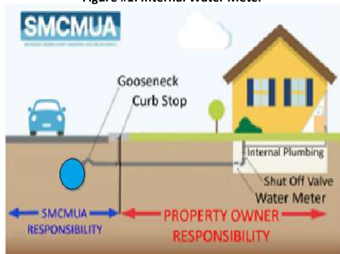
Figure #1: Internal Water Meter
